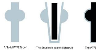
A Solid PTFE type t gasket is guaranteed to fail in SIP conditions. They will creep, cold flow and leak at ΔT. The Envelope gasket construction provides inconsistent results between the two materials. It will also creep, cold flow and leak over time. The PTFE grafted elastomer in a Tuf-Flex gasket will maintain I.D. without re-torquing or leaking.
